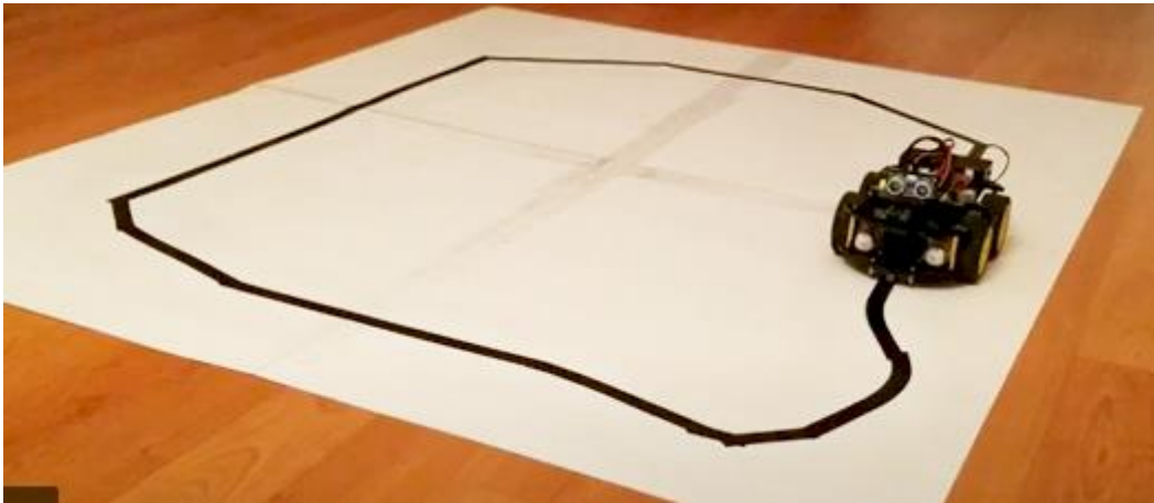
Fig. 6. Arduino robot in action – following a defined trajectory.
