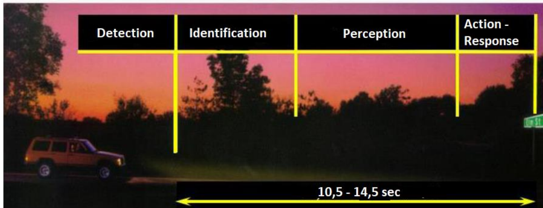
Image 2. The time it takes for a driver to be able to detect the sign and act on its interaction
